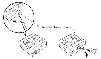
2. Connect the connection terminals of the Dual Charger units.
